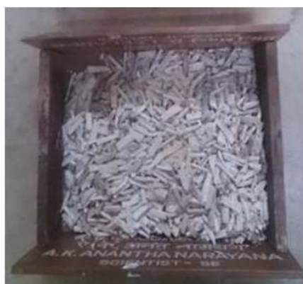
Figure 11: Wood Coated with Dolomite.
