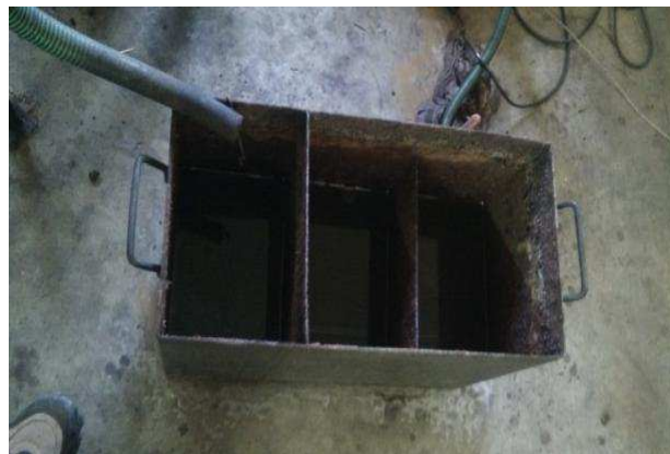
Figure 14: Recycling Water Tank.
