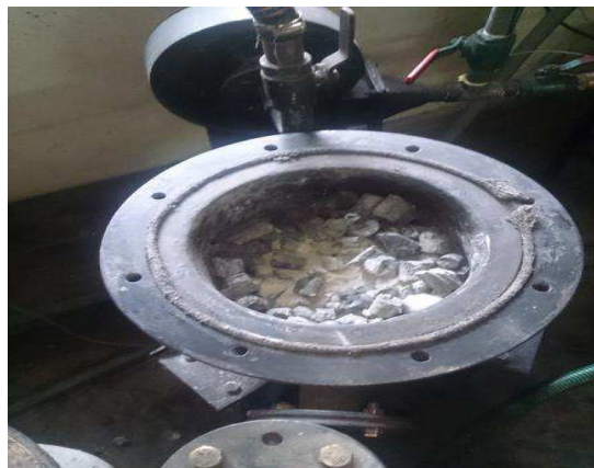
Figure 13: Reduction Zone of the Gasifier.
