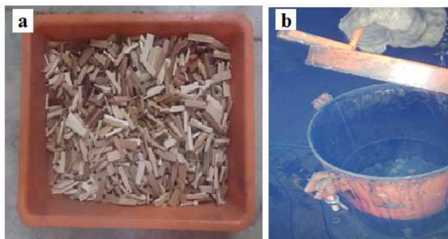
Figure 7: a. Wood Pieces of Approximate 5-10 cms in Size b. Gasifier Drum.
