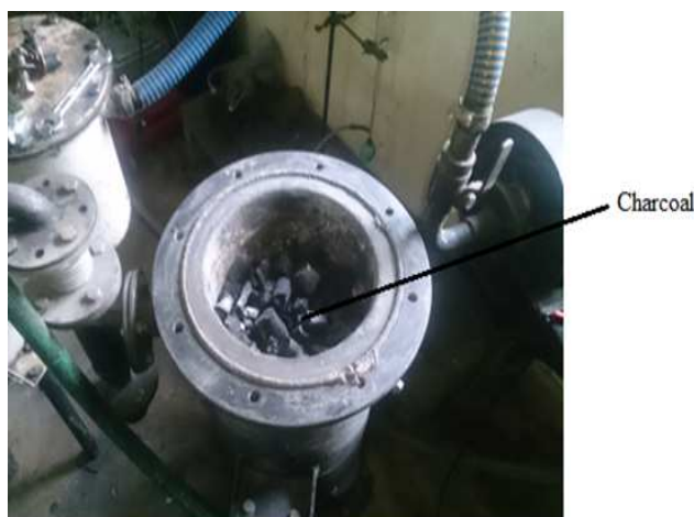
Figure 5: Charcoal Loaded in the Gasifier.
